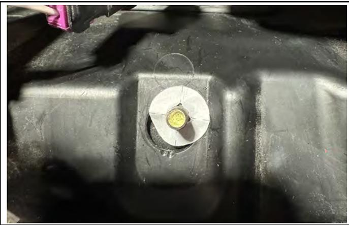
5. Using a paint pen, trace the outline of the template on the plastic of the under hood liner.
