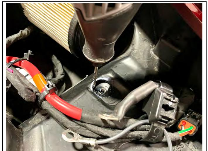
8. Debur the hole using a deburring tool.
